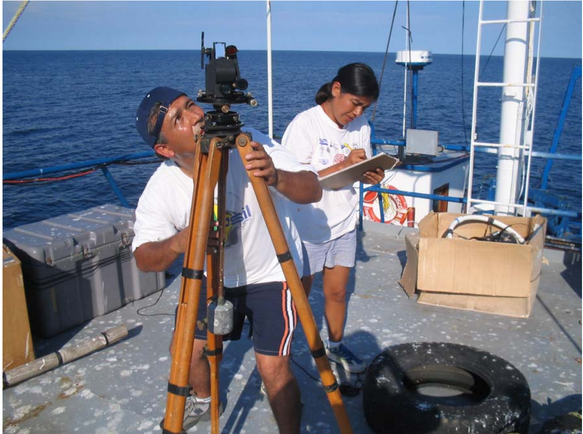
Figure 4. Theodolite on board the ship to track the meteorological balloons. Javier Murillo and Ana María Ramírez acquiring data.
