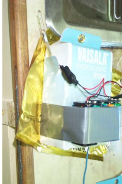
Figure 4. Vaisala radio probe system attached to the balloon for monitoring of meteorological variables in the lower atmosphere.
