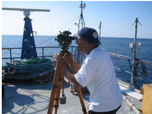
Figure 5. Theodolite on board the ship, to track the meteorological balloons.
