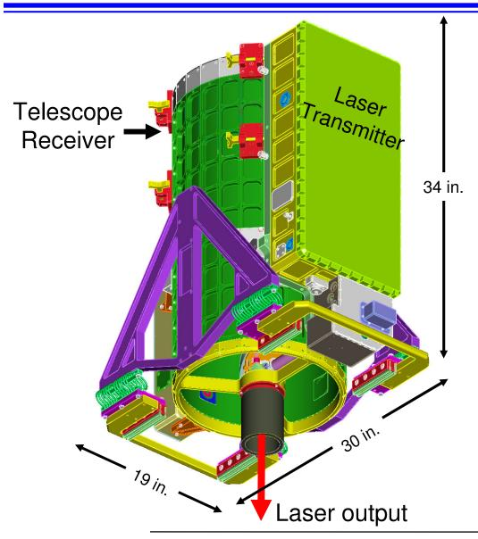
Independently measures aerosol/cloud extinction and backscatter at 532 nm
