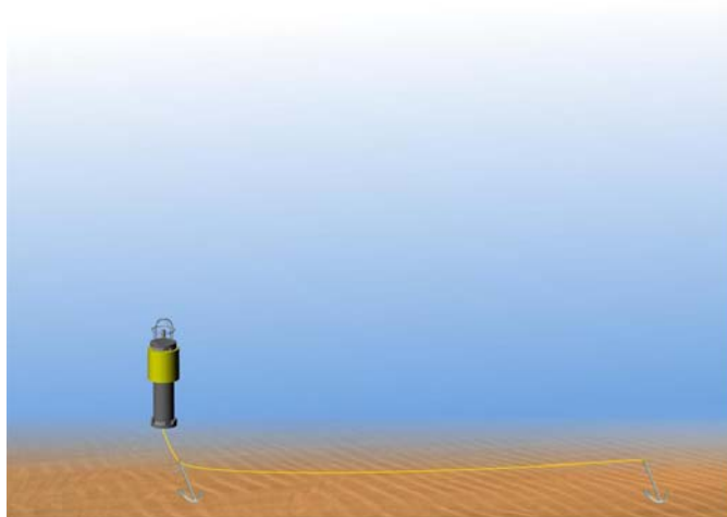
Figure VII-3: AMAR deployment configuration planned for CPAI 2009 acoustics program. Retrievals are made by grappling the line between the two anchors. This method has been used successfully in the previous Chukchi season programs and nothing is left on the seafloor.
