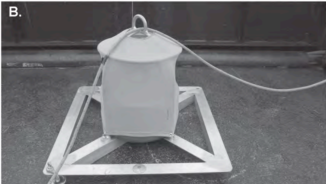
FIGURE X-2. DASAR recorder (model C08). (A) Schematic diagram of the components of the DASAR-C08 recorder. (B) A DASAR about to be deployed. The lowering line (shown) is looped through the top of the frame and is removed after the DASAR is set on the ocean floor. The ground line is attached with a shackle to the bottom left corner of the DASAR frame on the picture. At the end of its 110 m length, this line is connected to a chain and Danforth anchor, which are deployed last.
