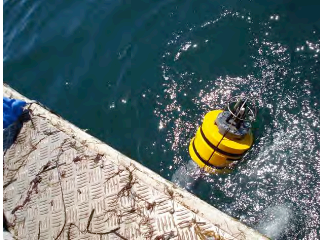
Figure IX-1. Photograph of AMAR acoustic buoy.
