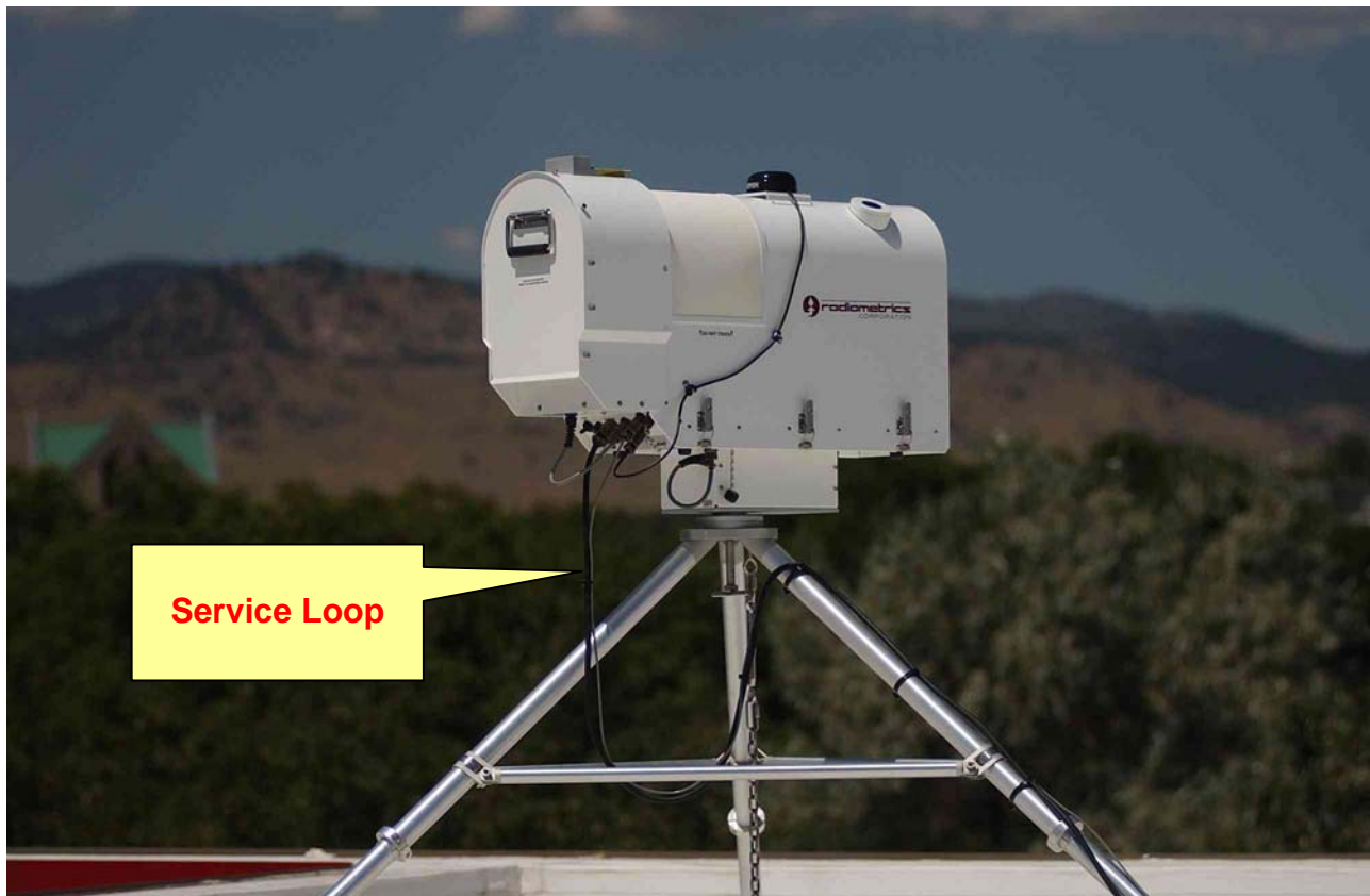
Figure 12 Cable service loop for use with Azimuth Positioner
