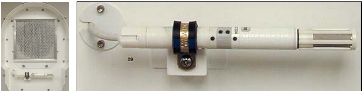
Figure 29 SuperBlower with End Cover removed; S3 sensor and filter.
