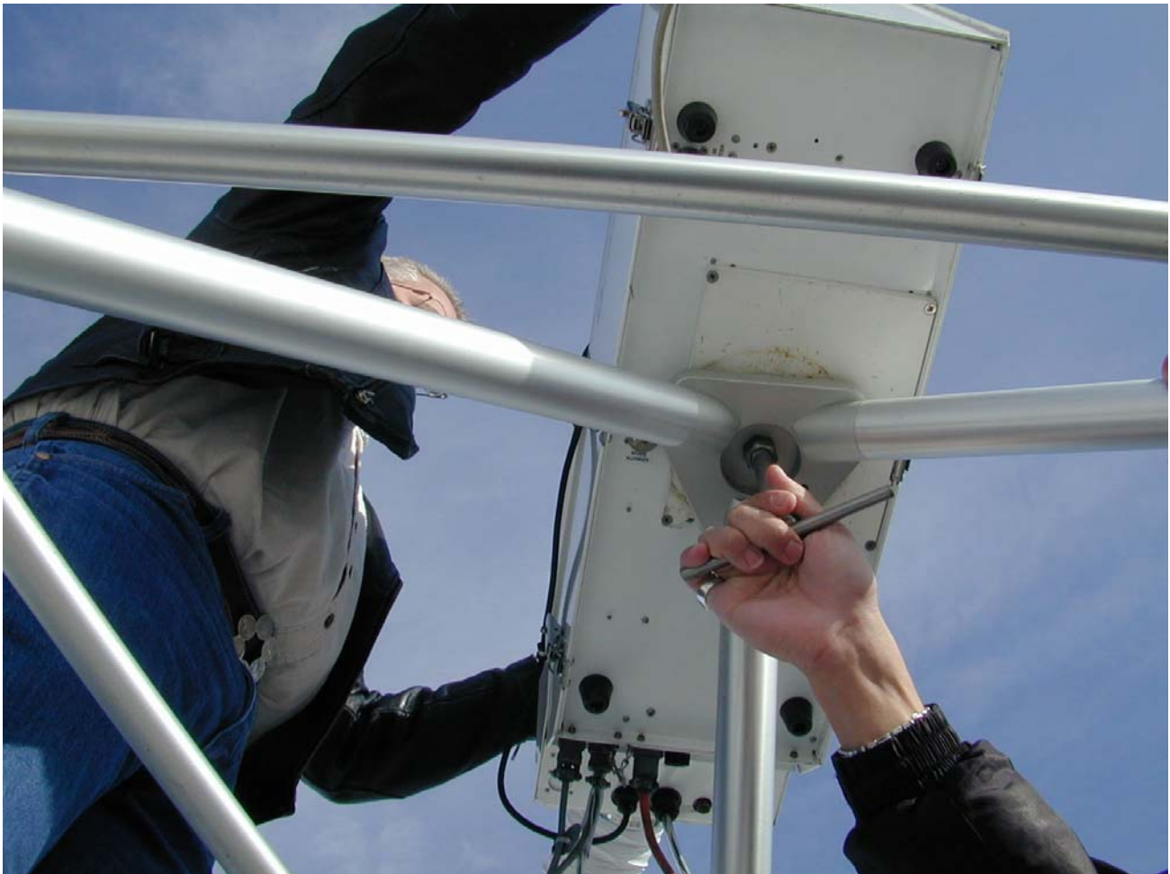
Figure 10 Securing the Profiling Radiometer with the T bolt
