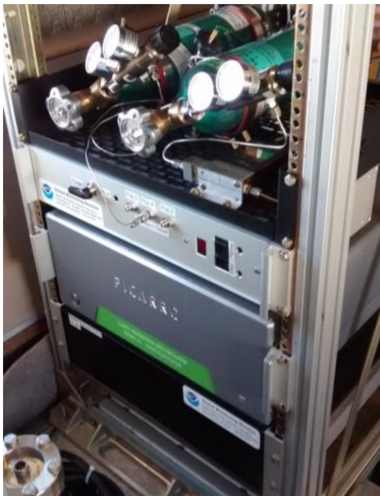
Figure 1. The NOAA Picarro system onboard the GV for the ORCAS campaign with the following modules from top to bottom: calibration tanks, valve box, analyzer, pump box.
