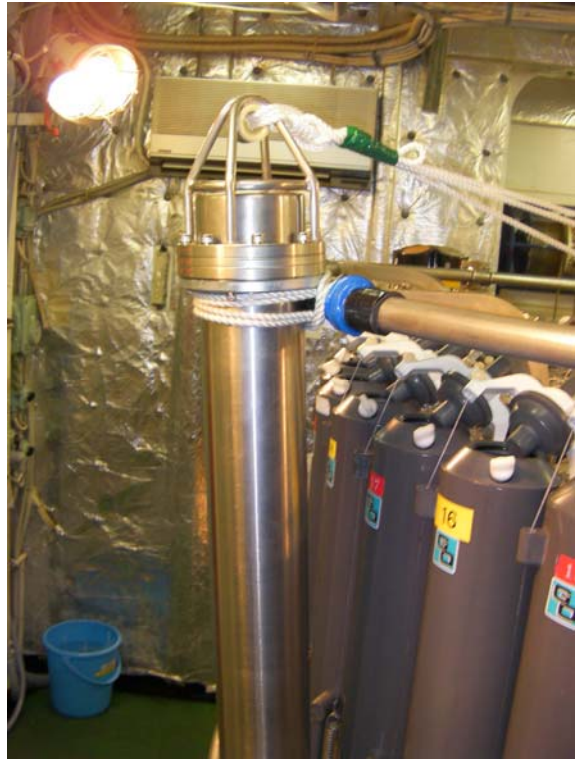
Figure 4.15-2. Acoustic release lashed to CTD frame for the response test of acoustic release in deep sea.
