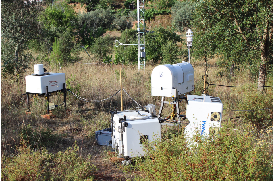
Figure 3: WC49 (lower Orange) with lid removed, view to south-southwest with other instrumentation (left to right): OU Halo, tower vall_04, and OU radiometer
