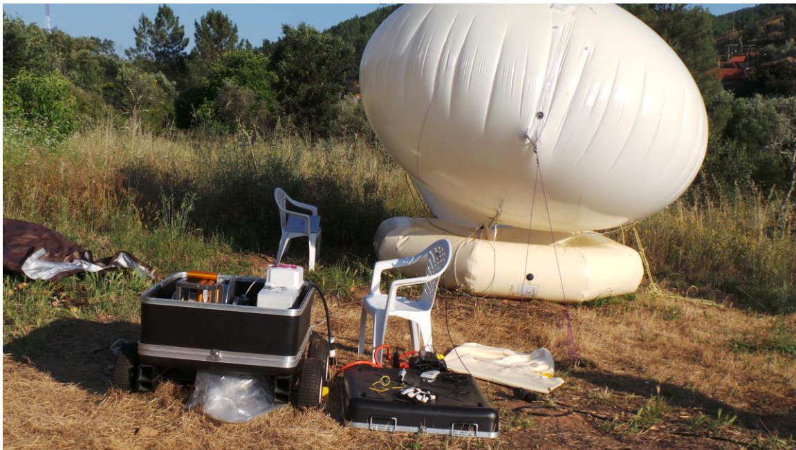
Figure 1: CU TLS with winch, helikite and base setup at lower orange site.
