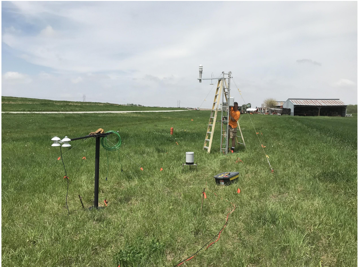
Figure 2: (from left) Hukseflux radiometer, surface rain gauge, and Vaisala PTB mounted at 2 m at the Roger's Farm site. This view is towards the north.
