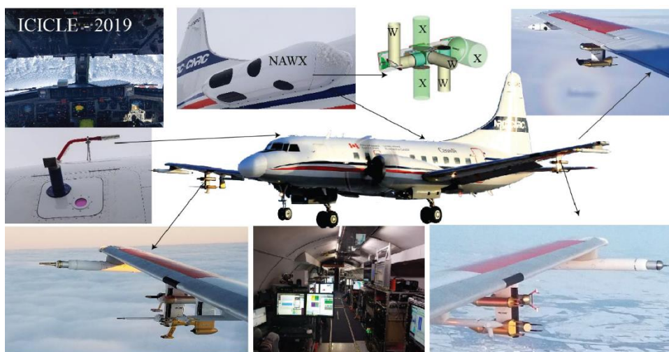
Figure 1 – A diagram of the Convair 580C instrumentation for the ICICLE campaign
