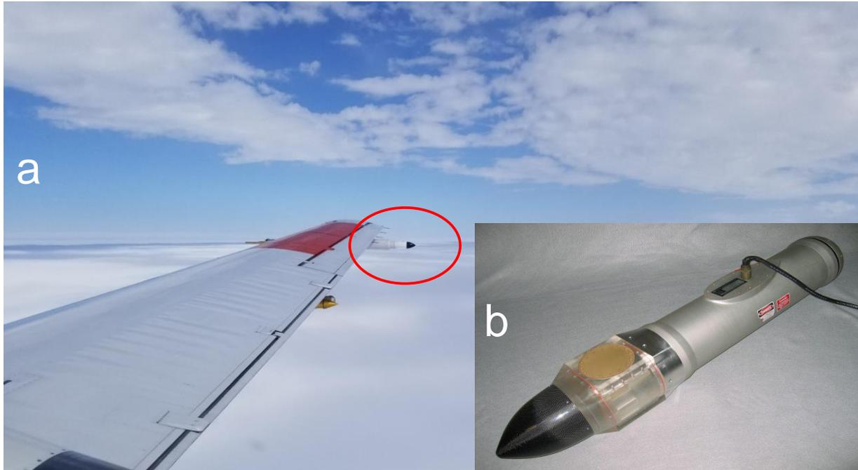
Figure 1. a) GVR installed in the starboard aft wingtip pod on the NRC Convair-580. Photo credit: NRC b) The G-band radiometer (GVR). Photo credit: ProSensing.
