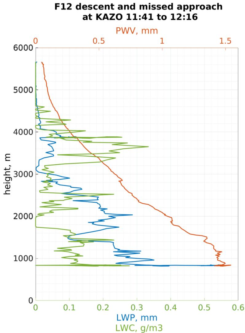
Figure 2b. Example of GVR pseudo-profile data during a missed approach at KAZO in Flight 12. Liquid water content (LWC) profile comes from Nevzorov probe (preliminary quality) data record.
