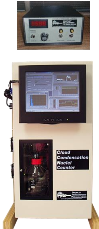
Figure 3. Cloud Condensation Nuclei Counter with Constant Pressure Inlet for airborne operation [3,4].
