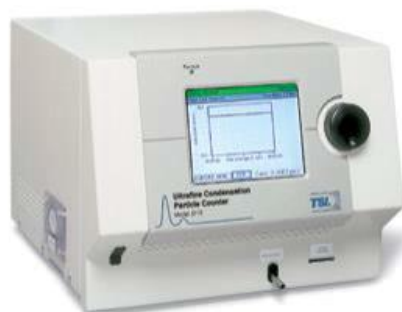
Figure 4. CPC 3775. Image by the manufacturer (TSI).
