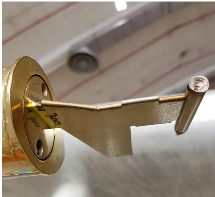
Figure 1. The Nevozorv, installed on NRC Convair-580 aircraft in starboard scalar boom (ssb) location.
