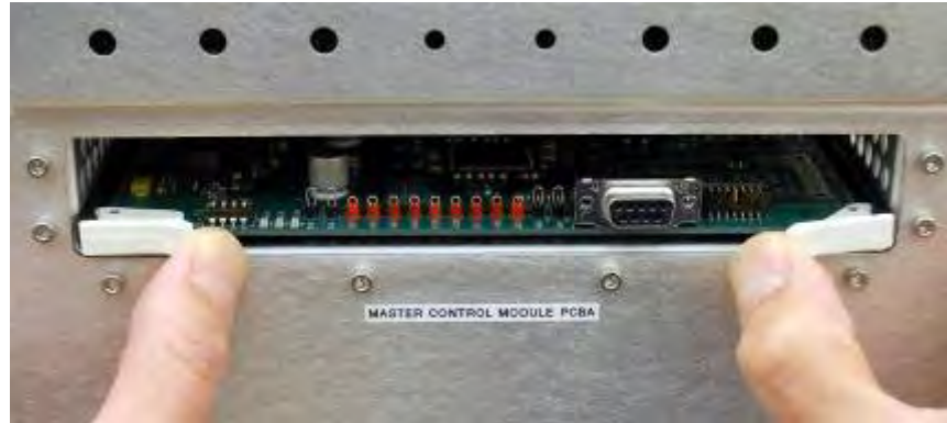
Figure G-12. Pulling release MCM PCBA latches
