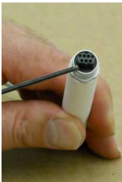
Figure G-28. HC2-S3 Ambient Air Probe, showing receptors
