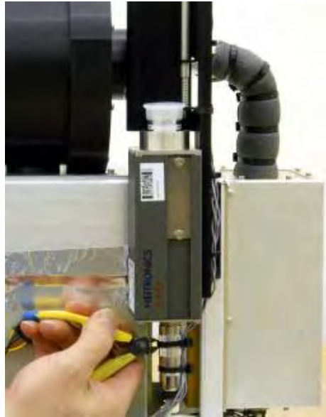
Figure G-5. Using wire cutters to remove cable-tie retainers
