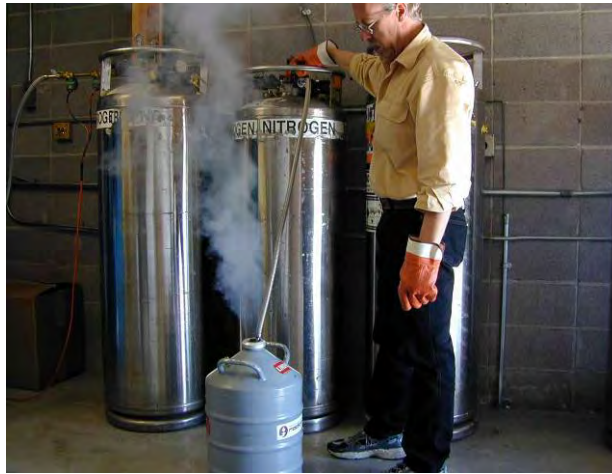
Figure E-10. Dewars used for storing and handling LN2
