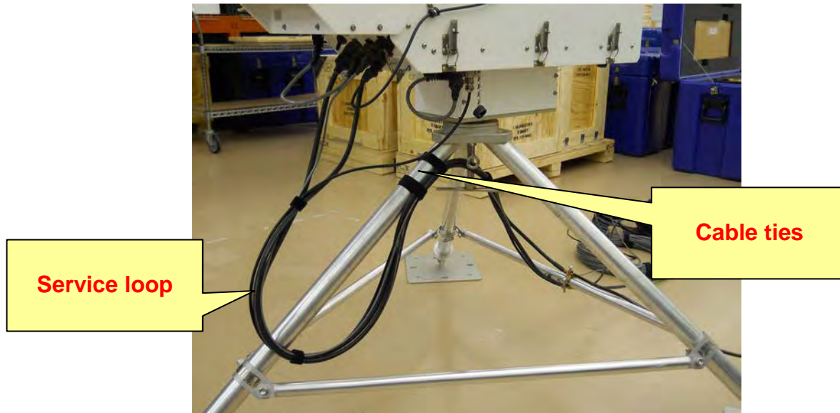
Figure 3-8. Cable service loop for use with Azimuth Positioner
