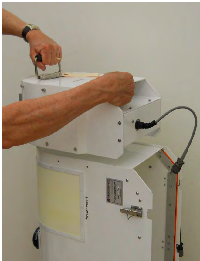
Figure G-35. Lifting Superblower away from the radiometer hood
