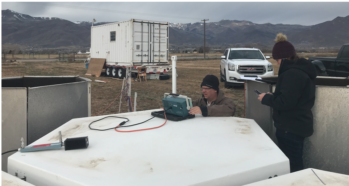
Testing the power amplifiers during the setup of the Modular Wind Profiler at CFACT.
