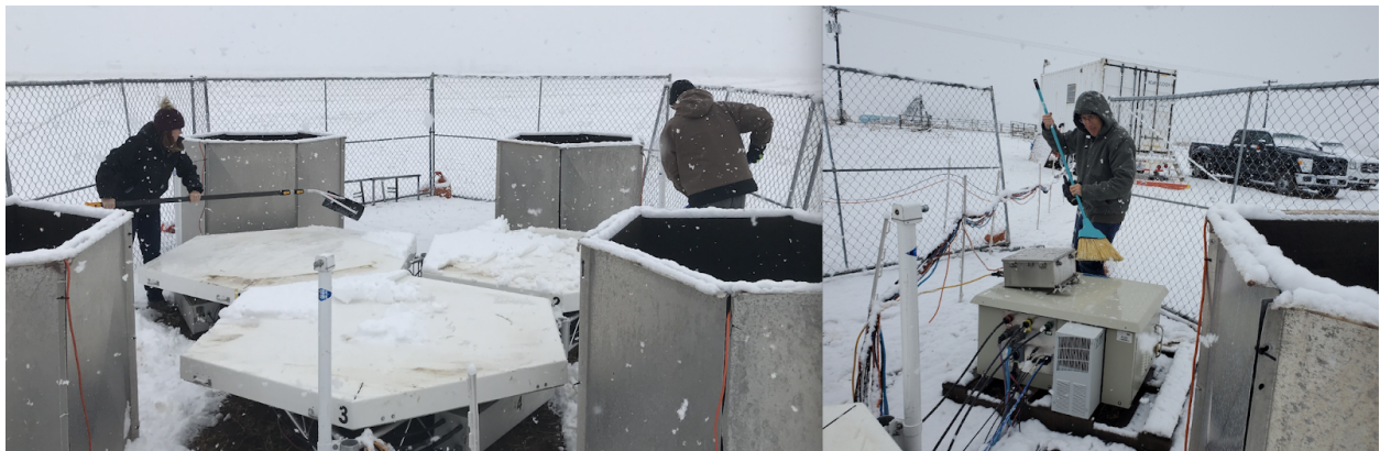
Clearing snow from the Modular Wind Profiler antennas and RASS dishes.
