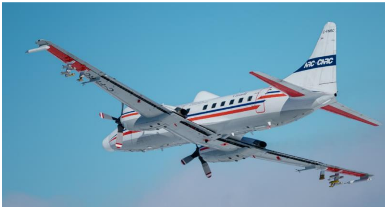
Figure 2. NRC Convair-580 research aircraft instrumented with underwing cloud probes.
