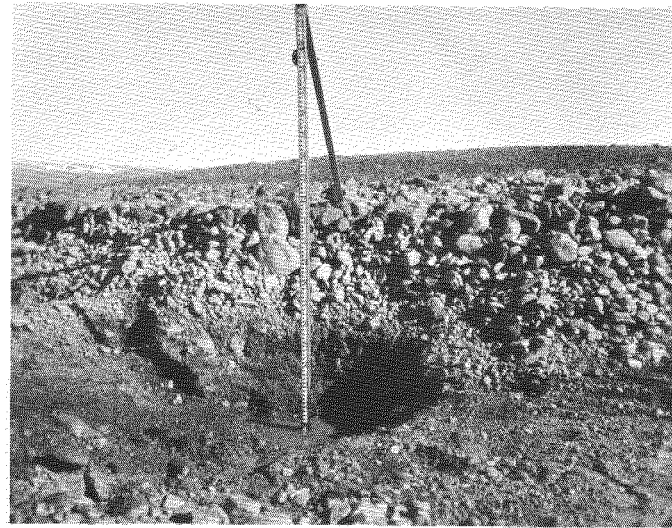
Fig. 6. Vertical sorting in the active layer at Thule, Greenland. The scale rests at 30 cm below permafrost
