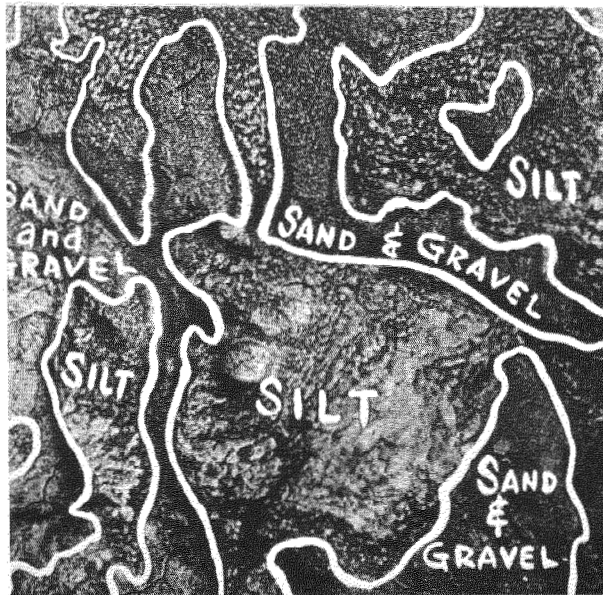
Fig. 5. Typical engineering soil maps prepared for site analysis in arctic areas
