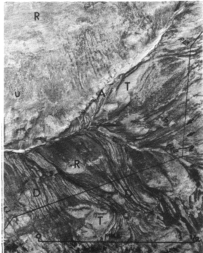
Fig. 2. Airphoto shows route location in vicinity of Mile 2. Letters are symbols for terrain conditions described in the text. Arrows point to localities of potential snowdrift. Grades are a major consideration in road location. Note distinctive gullies on terrain D
