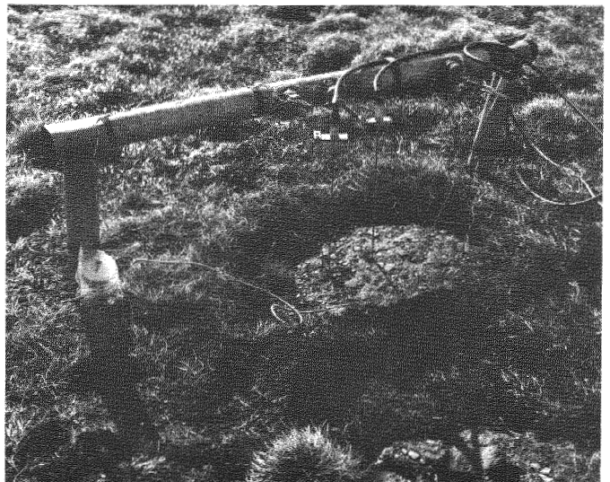
Fig. 2. Instrument emplacement in Northwestern Alaska, sites 1 to 3W. Movement is being recorded from different depths in a nonsorted mud circle
