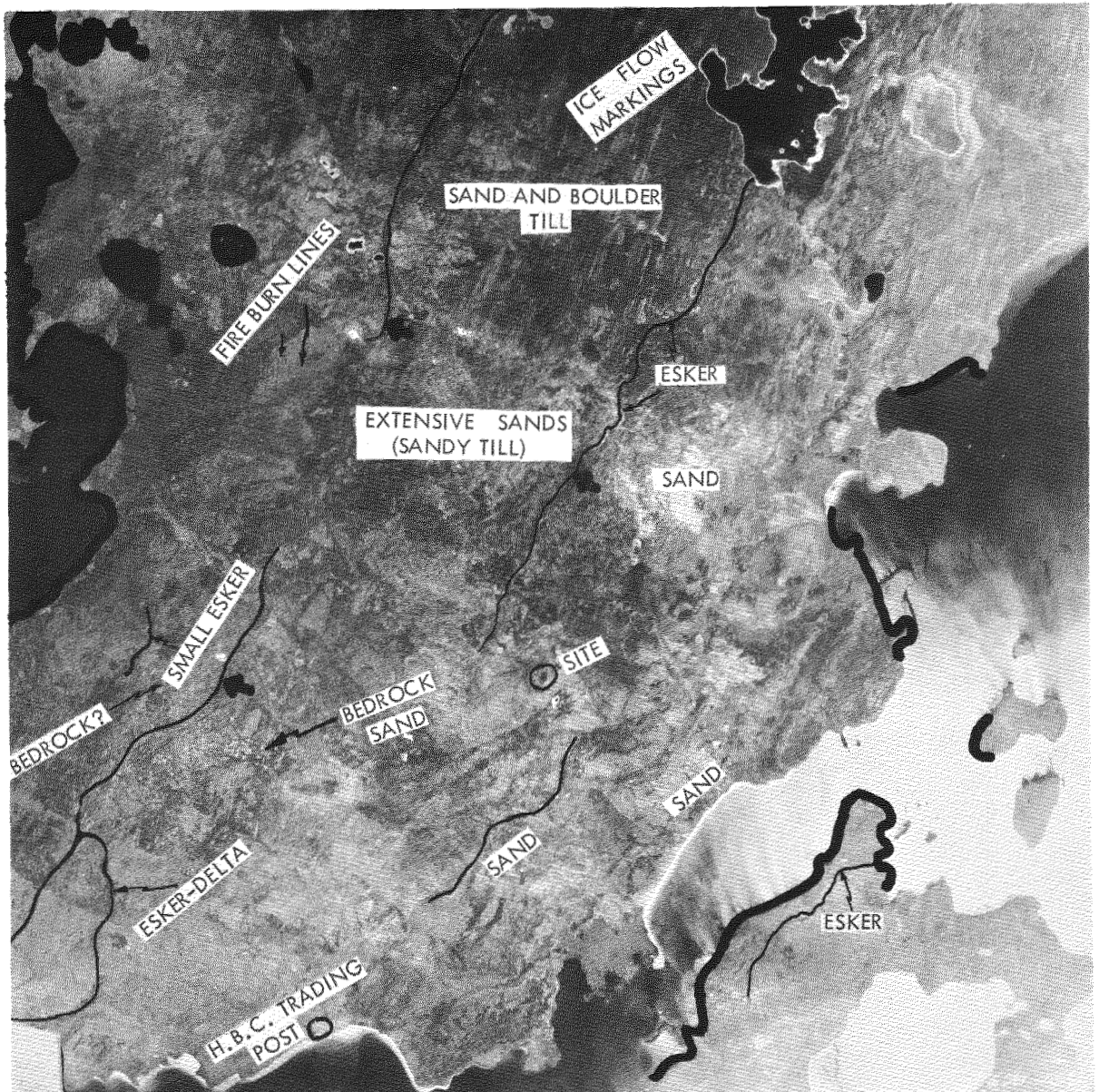
Fig. 6. Airphoto interpretation for construction materials in permafrost
