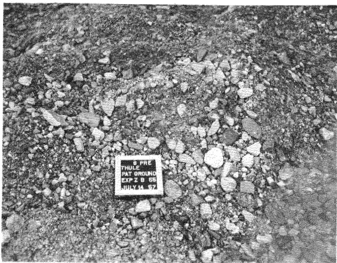
Fig. 2. Sorting produced experimentally after 44 days of melting by an uneven layer of gravel over glacier ice
