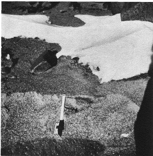
FIGURE 4 Soil of the trough of a well-developed, nonsorted polygon (Profile 39), Beacon Valley. The entire thickness of the soil above the ice-cemented permafrost is structureless, loose, noncoherent, and able to flow.
