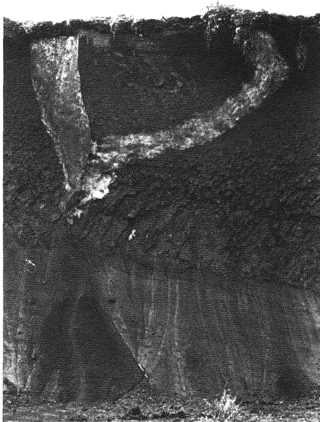
FIGURE 2 Slump section, about 8 m high, showing two ice wedges and stony clay (glacial till), with massive ground ice at the bottom. This is part of the ice shown in Figures 3 and 5. Location, 25 km southeast of Tuktoyaktuk, N.W.T.
