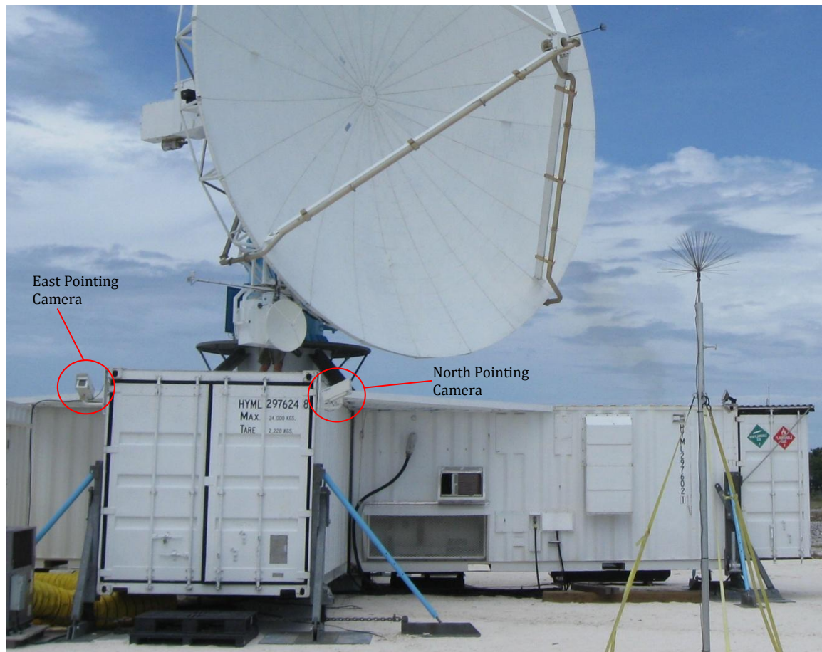
Figure 1: Photo showing cameras mounted on the east-pointing container of the main S-PolKa structure. A similar arrangement appears on the west-pointing container for the south- and west-pointing cameras.
