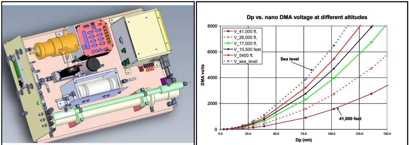
Figure 1 (left): The EC shown on HIAPER shelf (tubing and filter cover removed for clarity); (right) GV SMPS particle size/voltage relationship
