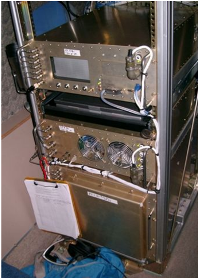
Figure 1. The AO2 system as used during HIPPO flights on the NSF/NCAR GV. The instrument module is on top, the pump module in the middle, and the cylinder module on the bottom. The dewar, line purge cylinder, and inlet pressure controller are not shown.
