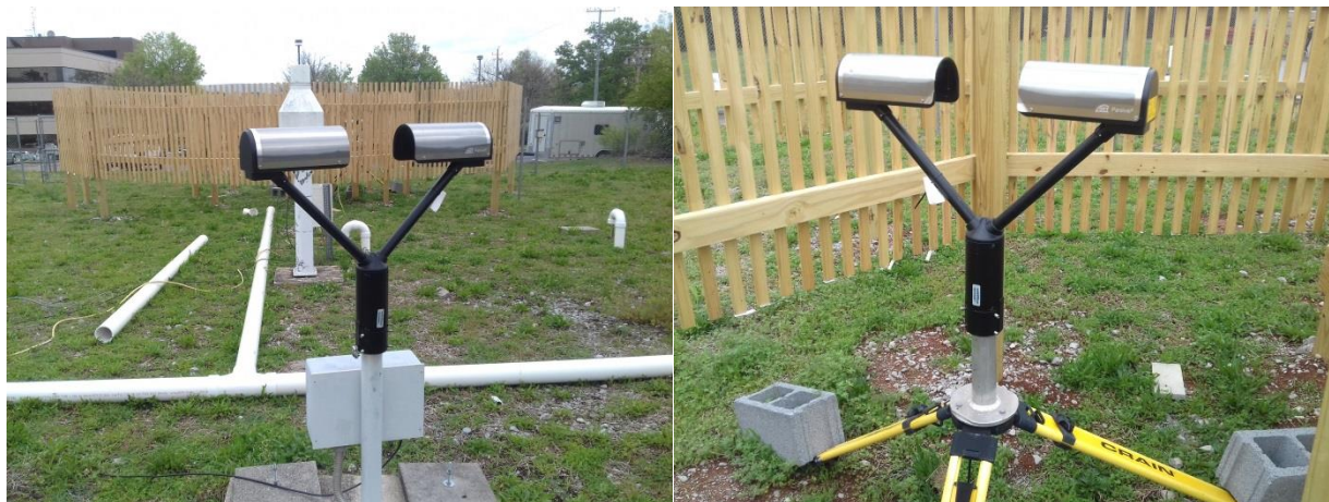
Figure 1 – Left: Outside-fence Parsivel disdrometer and the fence on the back. Right: Inside-fence Parsivel disdrometer.
