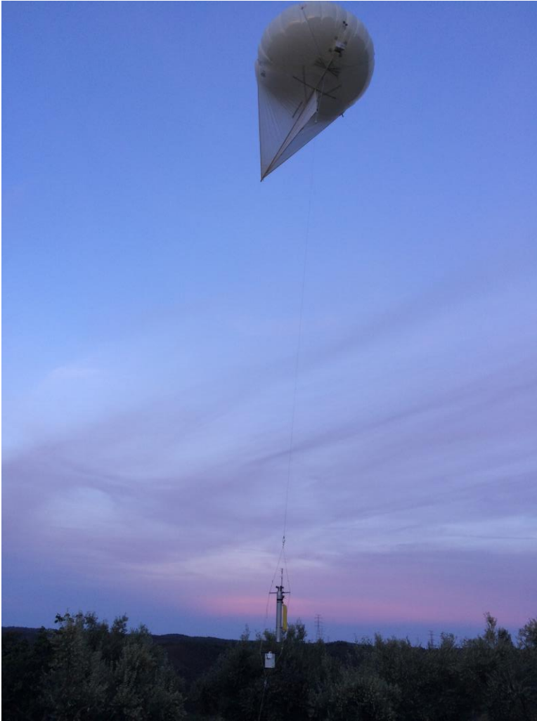
Figure 2: ARL TLS with suspended turbulent payload in profiling mode.
