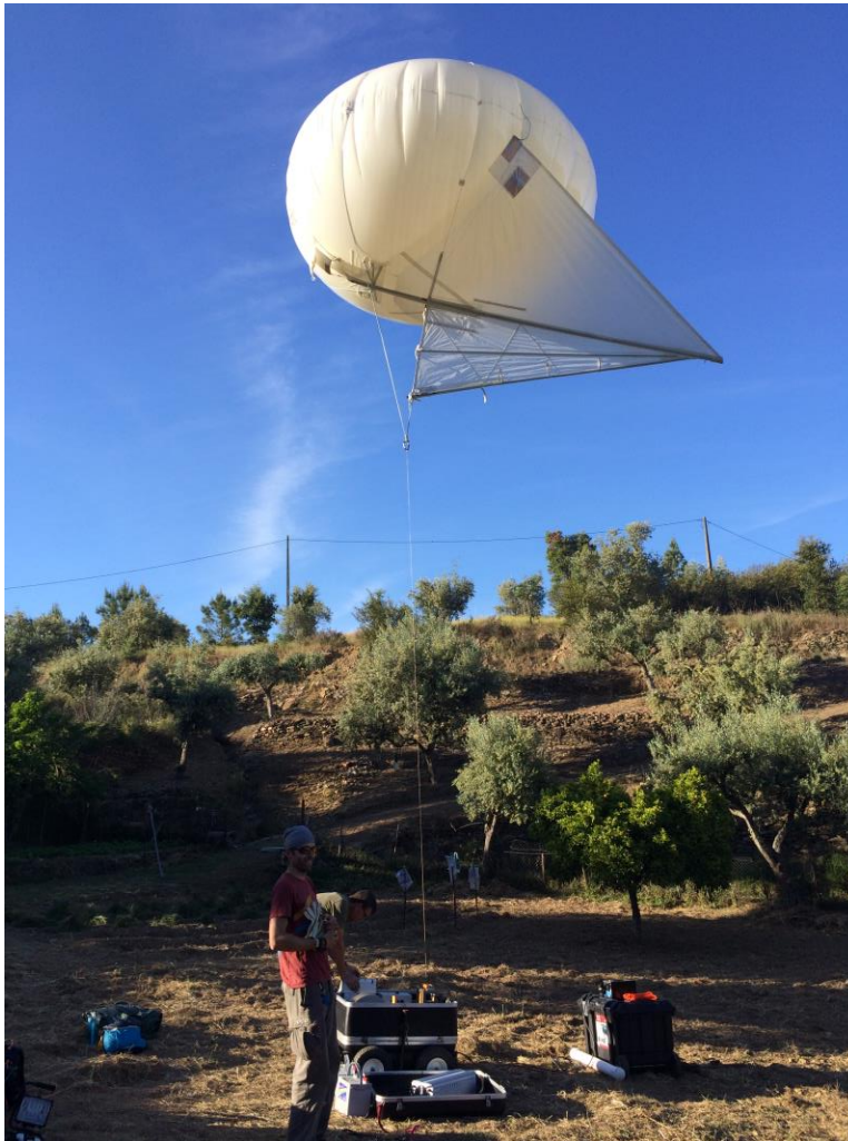
Figure 1: ARL TLS with winch, helikite and base setup at 'George' site.
