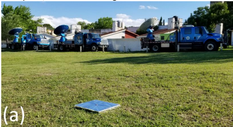
Photograph of hail pad in front of the Doppler on Wheels radars. Taken by M. Kumjian.
