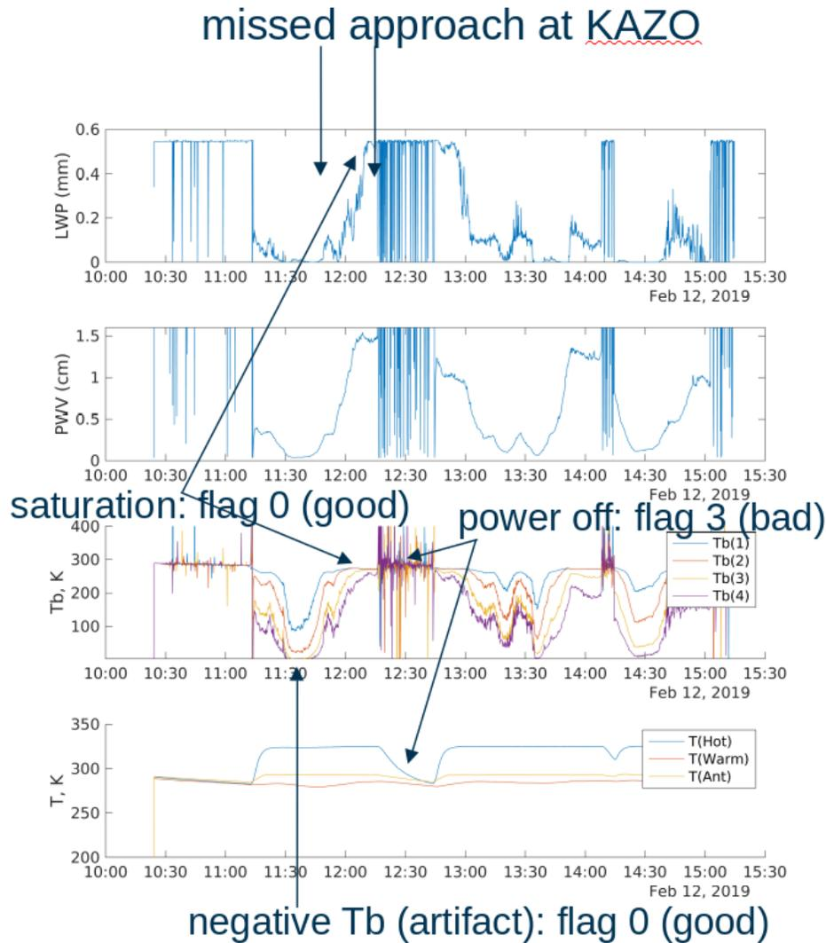
Figure 2a. Example of GVR data during Flight 12 of ICICLE with possible issues labeled.
