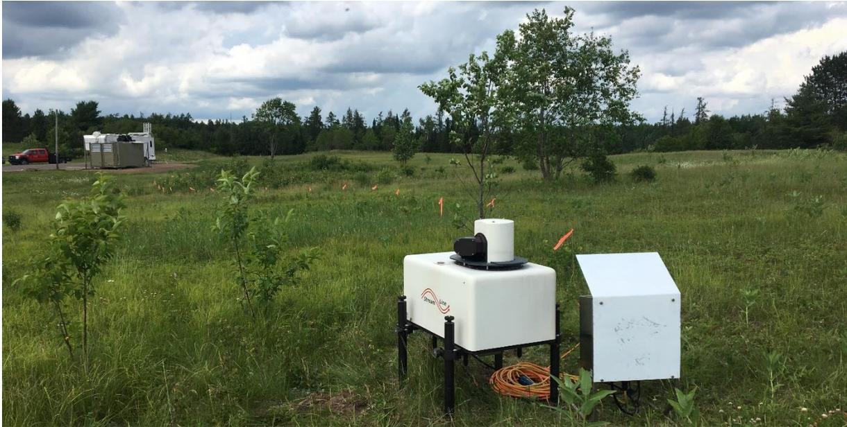
Figure 2: Halo Photonics Stream Line Doppler LiDAR at the CHEESEHEAD measurement campaign
