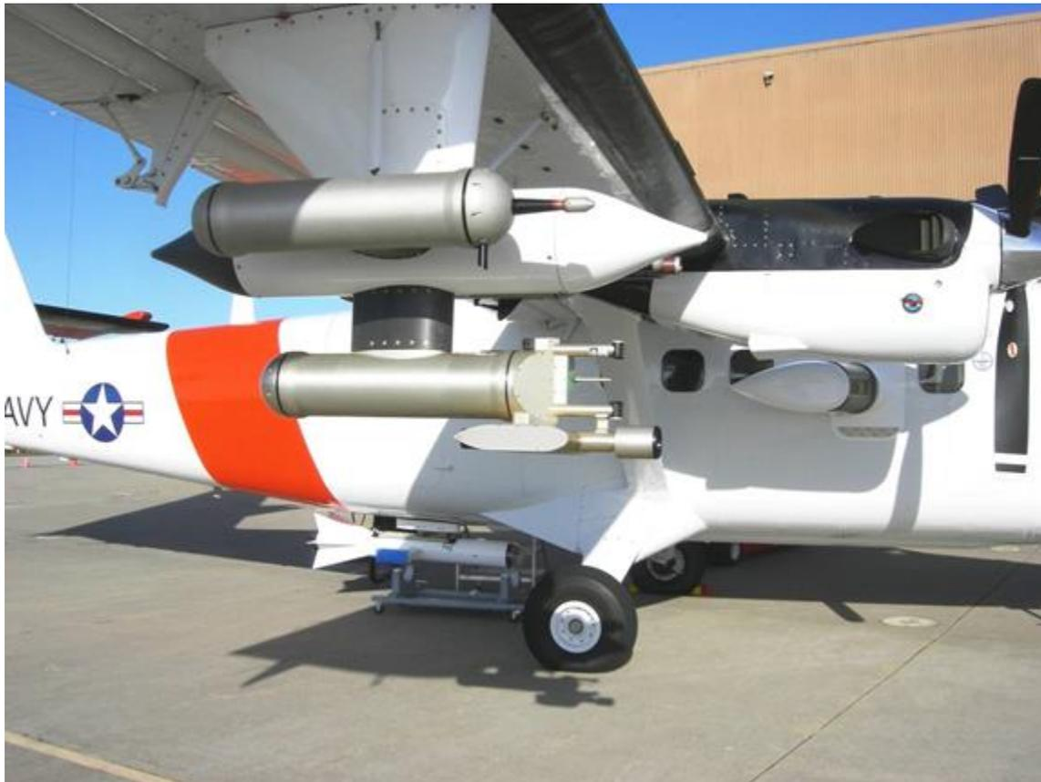
Figure 1: TODWL on board a Twin Otter aircraft
