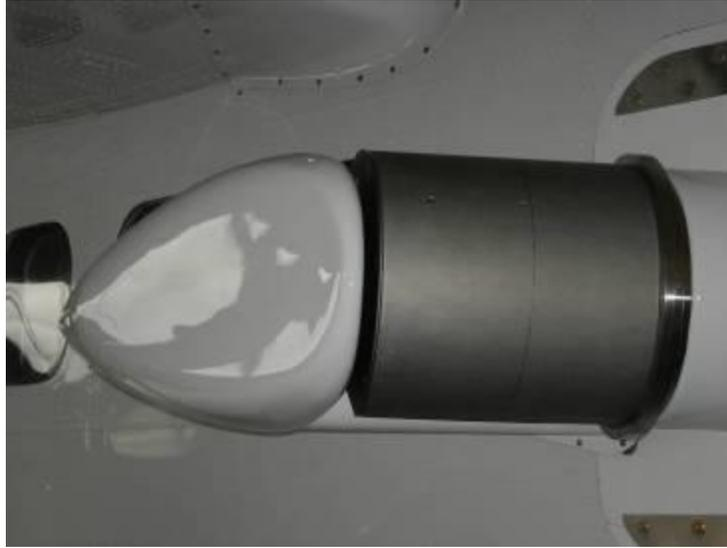
Figure 2: Close-up of TODWL scanner on board a Twin Otter aircraft
