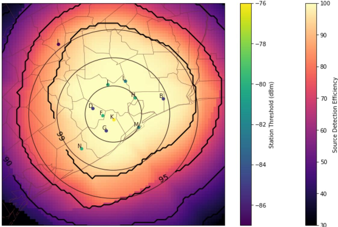
The figure above shows the estimated (method of Chmielewski and Bruning, 2016) flash detection efficiency (black contours) source detection efficiency (purple-yellow shading) and the location and receiver threshold at each LMA station, indicated by their letter codes. Range rings from the CSAPR radar are shown at 50, 100, and 150 km.
