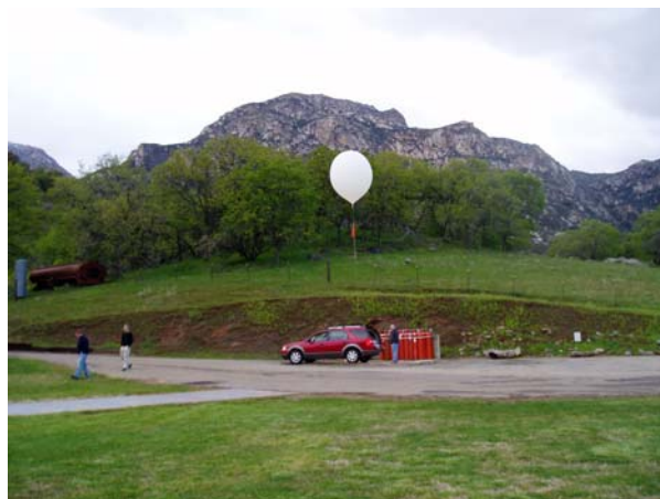
Figure 2. Radiosonde ready for launch near helium tanks on the northern edge of the Ash Mountain Helibase. The ridge shown behind the balloon frequently blocked radio signals from radiosondes that began their flight heading northward.
