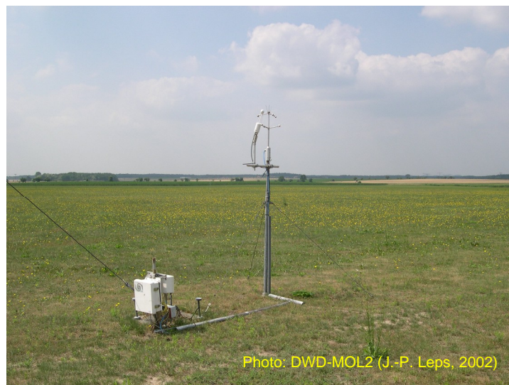
Figure 10 Turbulence measurement system S1 (USA-1 sonic + LI7500 hygrometer)
