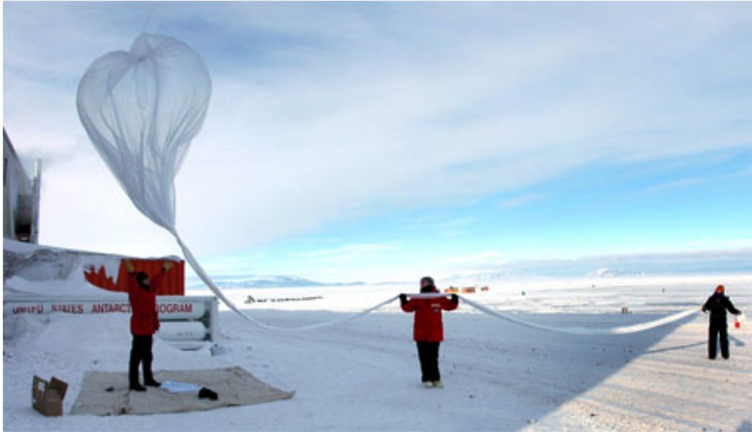
Figure 1 Deployment of a stratospheric balloon during CONCORDIASI, 2010 (Photo: Philippe Cocquerez).
