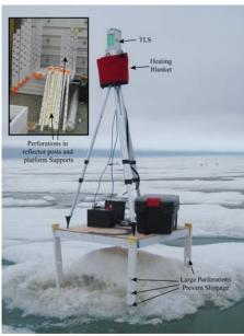
LiDAR Scanner on custom platforms Inset: reflectors prior to installation
