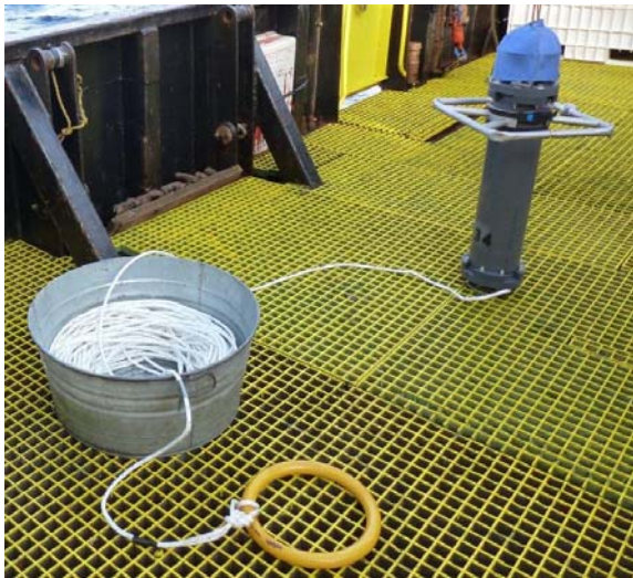
Figure 3. An AMAR being deployed from the M/V Westward Wind in summer 2011 in the northeastern Chukchi Sea.
