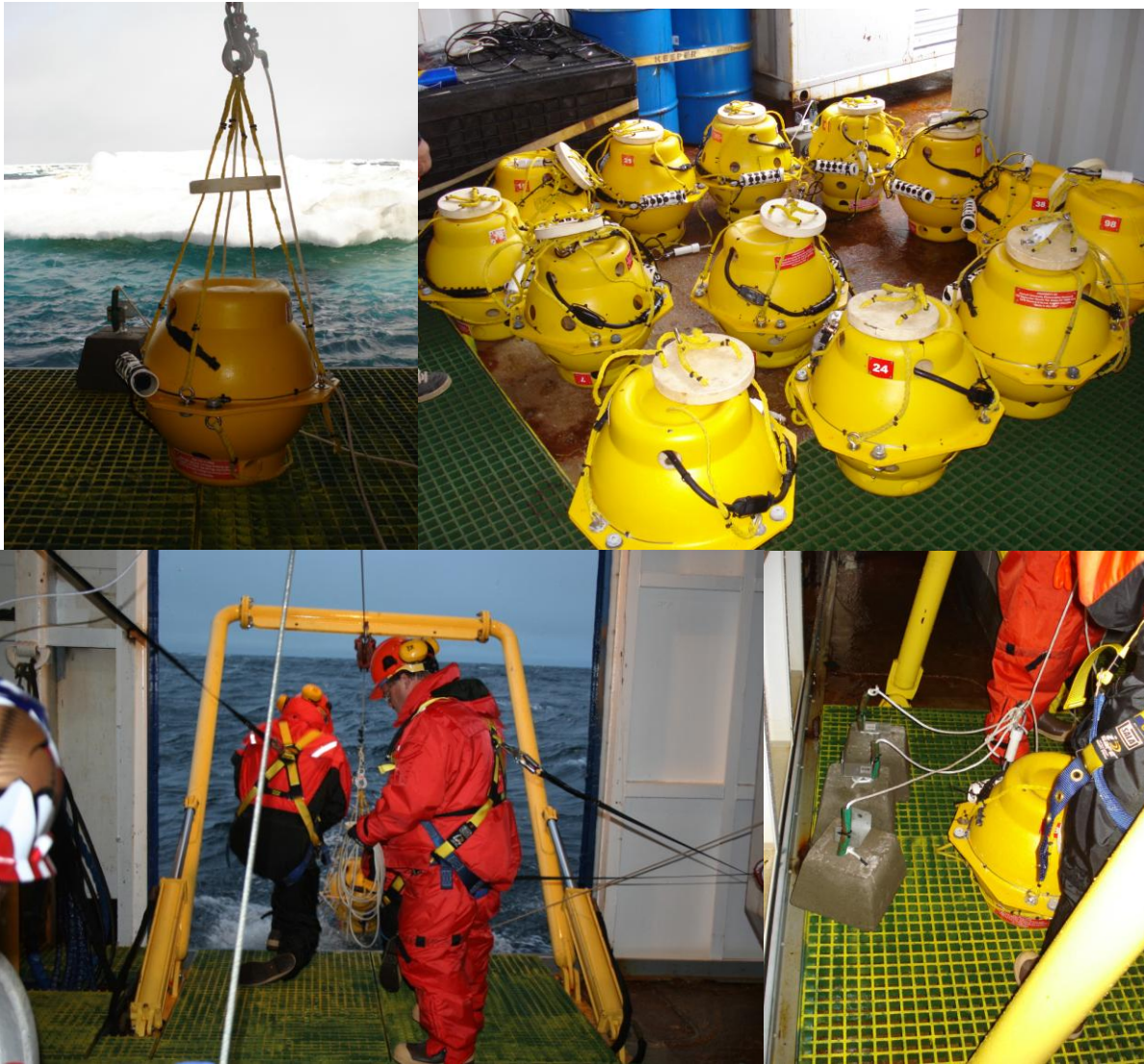
Figure 1. Deployment of Marine Autonomous Recording Units (MARUs) in the Chukchi Sea, summer 2008.
