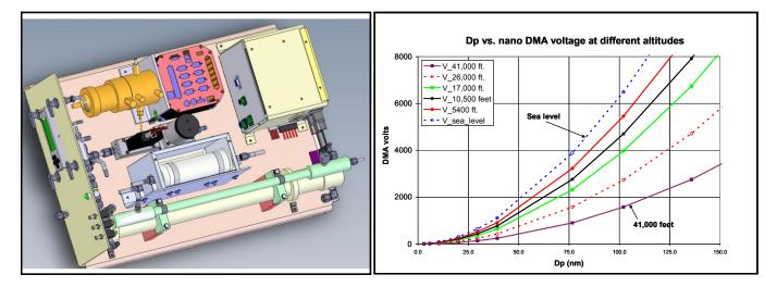
Figure 1 (left): The EC shown on HIAPER shelf (tubing and filter cover removed for clarity); (right) GV SMPS particle size/voltage relationship
