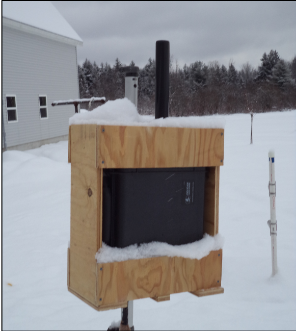
The HYVIS snow crystal imager, mounted on a tripod using a wooden frame.
