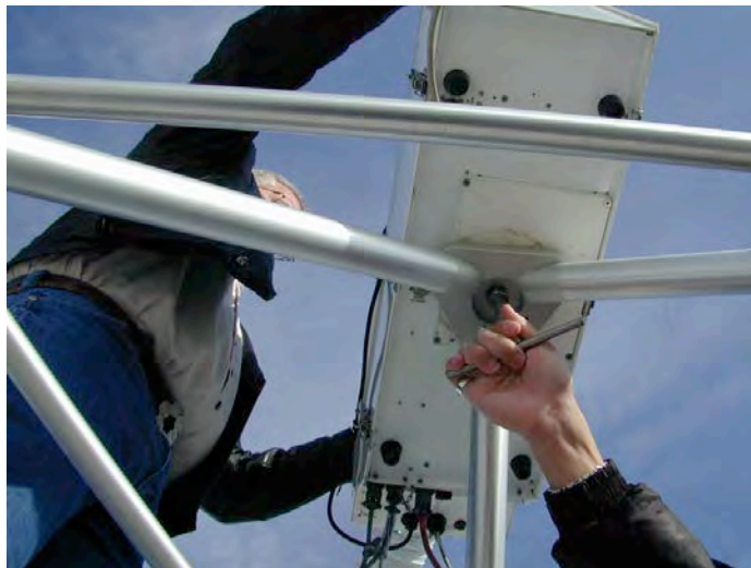
Figure 3-4. Securing the profiling radiometer with the T-Bolt
