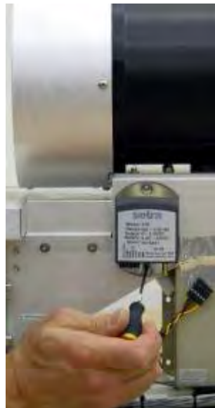
Figure G-31. Detaching Pressure Sensor from its frame
