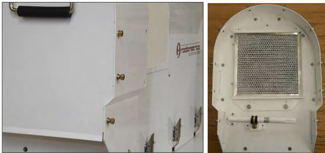
Figure G-26. Loosened thumbscrews on Superblower cover; cover removed (right)
