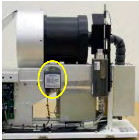
Figure G-29. Pressure Sensor on right side of radiometer
