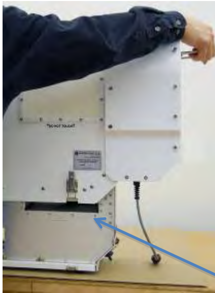
Figure G-10. Removing radiometer hood to reveal MCM PCBA
