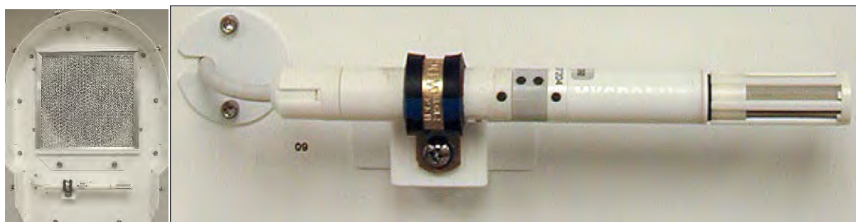
Figure E-14. Superblower with End Cover removed; sensor and filter
