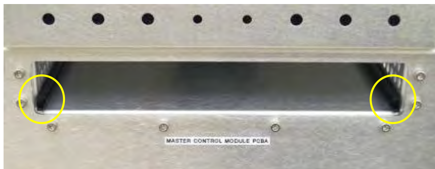
Figure G-13. Empty card cage, showing card rails
