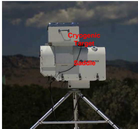
Figure E-2. Radiometer with Saddle and Cryogenic Target in place
