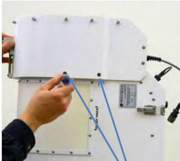
Figure G-34. Removing Superblower screws (two on each side)
