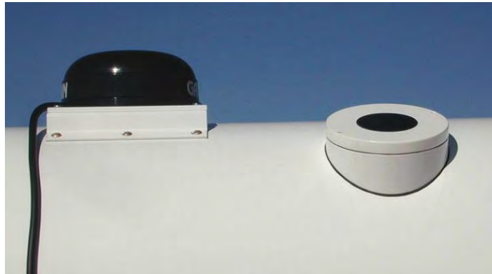
Figure 6-9. GPS Receiver on the left; IRT window on the right
