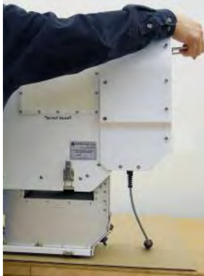
Figure G-2. One person, lifting the radiometer hood straight up
