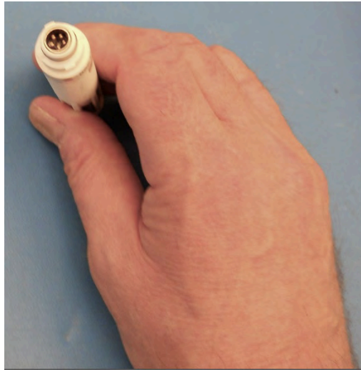
Figure G-25. S3 Temperature and RH Sensor, showing receptors
