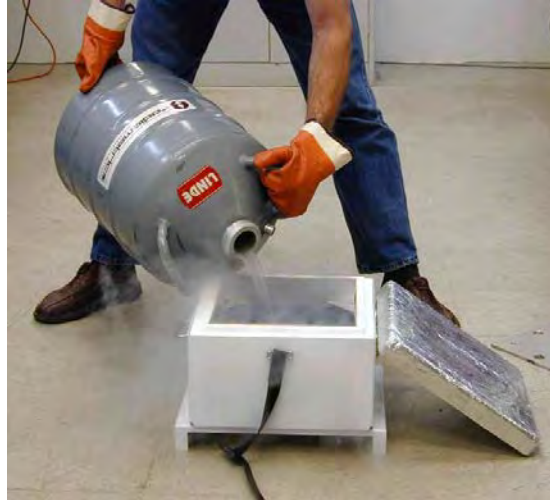
Figure E-4. Proper method for safely pouring LN2 into the Cryogenic Target
