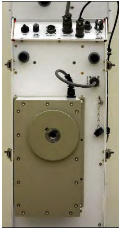
Figure H-2. Underside of radiometer with Azimuth Drive installed
