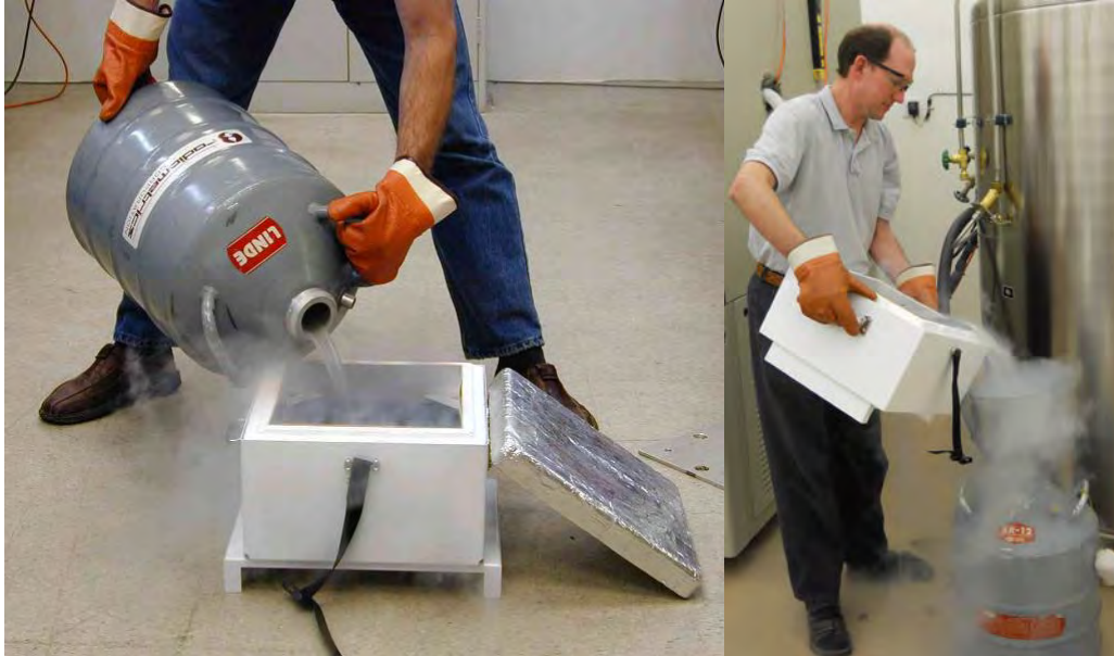
Figure D-11. Handling LN2: filling Cryogenic Target (left), pouring residual LN2 into Dewar after calibration is finished (right)
