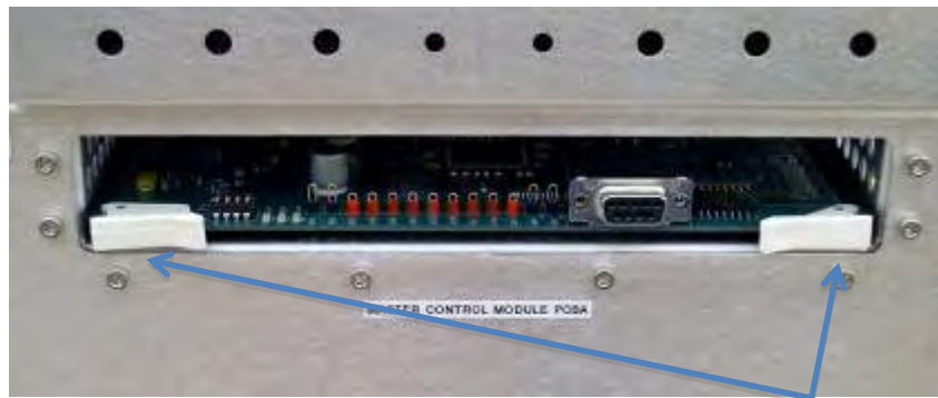
Figure G-11. Close-up view of MCM PCBA, with two plastic latches
