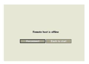
If connection is problematic, check that your attached PC is using the correct network settings and that the correct RJ connection and leads are being used. If the problem persists, follow this procedure:
