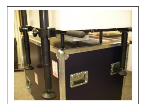
The LiDAR can now be lifted off and gently placed onto the floor. It will be necessary to support the LiDAR while the last leg is attached.
