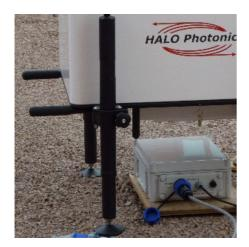
It is recommended that the power supply module be located directly underneath the LiDAR, and raised off the ground to reduce exposure to the weather. The module's enclosure is rated to IP66, but minimising exposure to the weather will only help.
