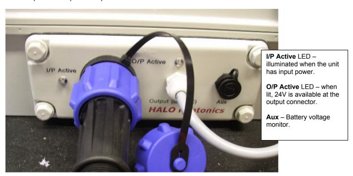
The module will provide a 24V DC output for approximately 30 minutes after input power is lost. The LiDAR software will shut the system down gracefully to minimise the risk of damage to the internal hardware and software when the voltage from the module falls to 20.5V or below. This auto shutdown is only active while the LiDAR main control software is running and the LiDAR is taking data.
