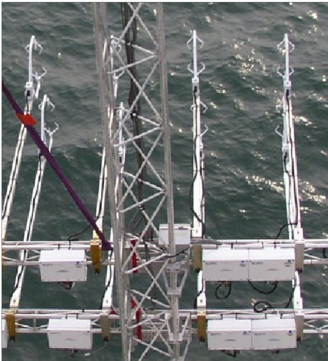
Figure 4. MotionPak (small gray box) mounted on upper (5.6 m) sonic array.
