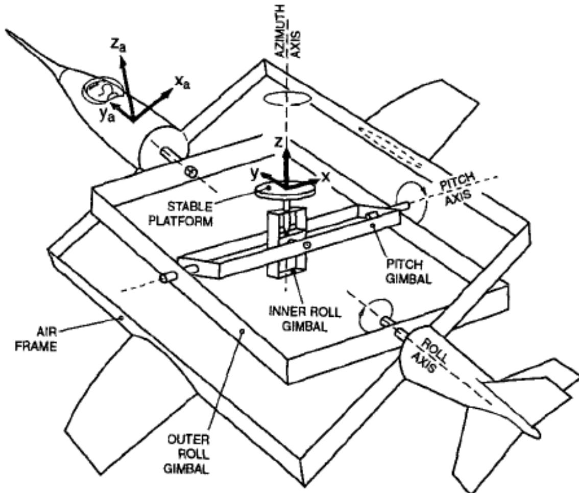
Figure 5.1: Moving platform axis definitions and reference frame
