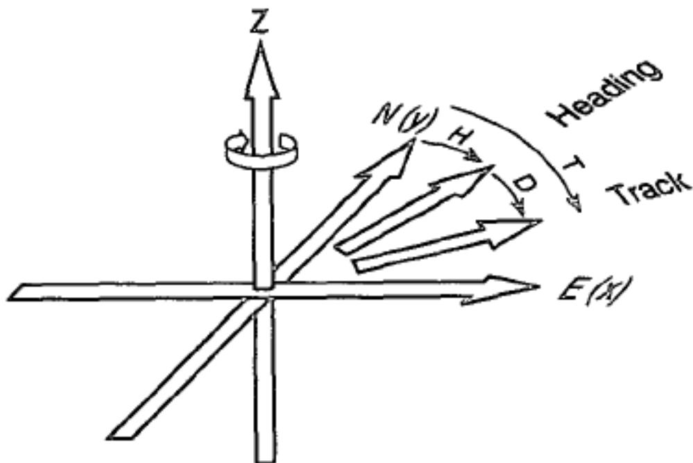
Figure 5.2(a): Definition of heading, drift and track.
