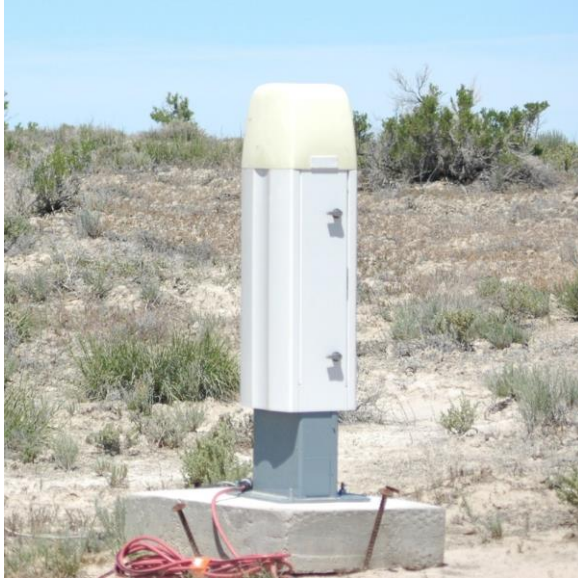
* This is a photo of the NWG Ceilometer, it is used here to depict a CL31
