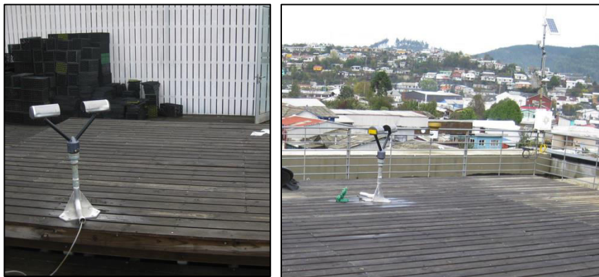
Figure 2: Photos showing the Parsivel as deployed at CRL
