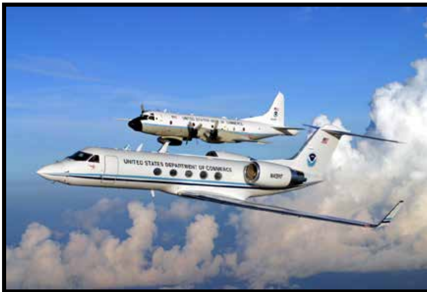
Figure 5-2. NOAA G-IV and WP-3D Weather Surveillance/Hurricane Aircraft
