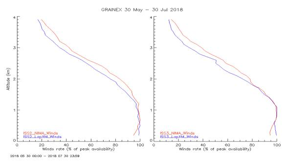
Winds height coverage profiles for the whole project, showing LapXM (blue) and NIMA (red). NIMA returns approximately an extra 200m at the 75% level (about 2.2 km for NIMA, 2.0 km for LapXM) at both sites. These profiles are normalized so don't reveal gaps in time.
