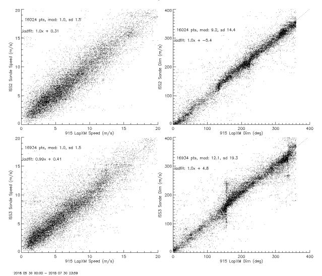
Profiler LapXM winds verses soundings for both sites and both IOPs for each height bin (instead of being averaged). Good agreement, although the ISS3 profiler wind directions have an artifact, particularly near the southerly direction. Ground clutter is suspected to play a role in this artifact.
