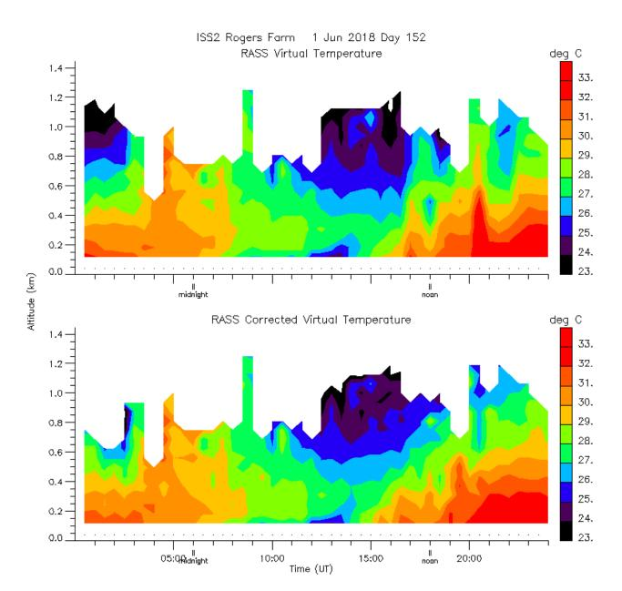
RASS virtual temperature measurements for the same day. Daytime boundary layer heating can be seen from about 16 UTC, although the RASS range does not extend the full depth of the boundary layer beyond mid-morning. A slight inversion can be seen after midnight at the 200 - 300 meter level.
