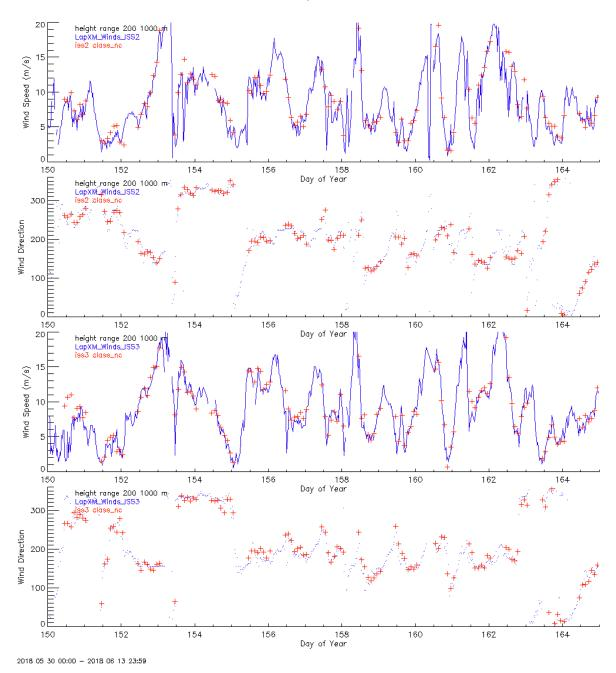
IOP #1 winds for both sites (averaged from 200m to 1km). Good agreement overall between soundings (red) and profiler winds (blue). Winds were slightly stronger at ISS3 (York, median 8.3 m/s) compared with ISS2 (Lincoln, median 7.8 m/s).
