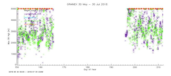
Wind availability in terms of max height coverage from the profilers (crosses - green for York ISS3 and blue for Lincoln ISS2) during the two IOP periods. The max coverage is slightly higher at the Lincoln site (median 3.1km) compared with the York site (median 2.9km). Max coverage is also a little higher for the second IOP. The red pluses indicate soundings.
