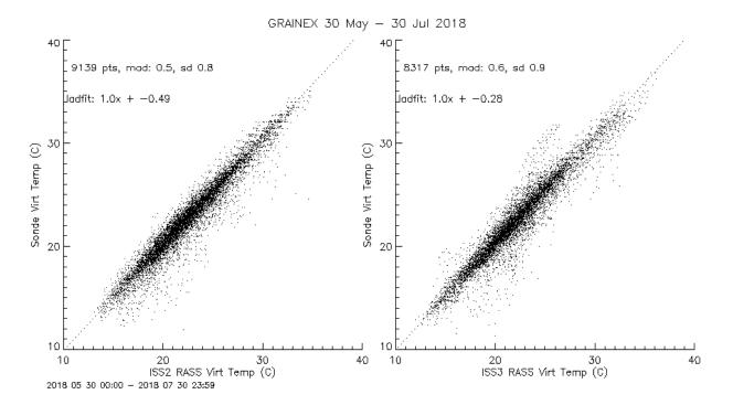
Comparison of RASS virtual temperatures from NIMA processing and from the soundings. The median absolute deviation is around 0.6 C and the standard deviation is around 0.9 C.
