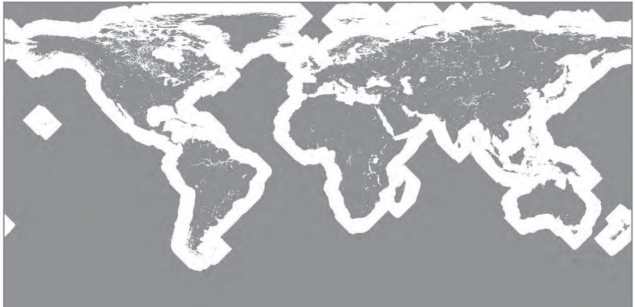
Figure 15. The SMAP high-resolution radar data will be collected one swath width across coastlines of continents and major islands
