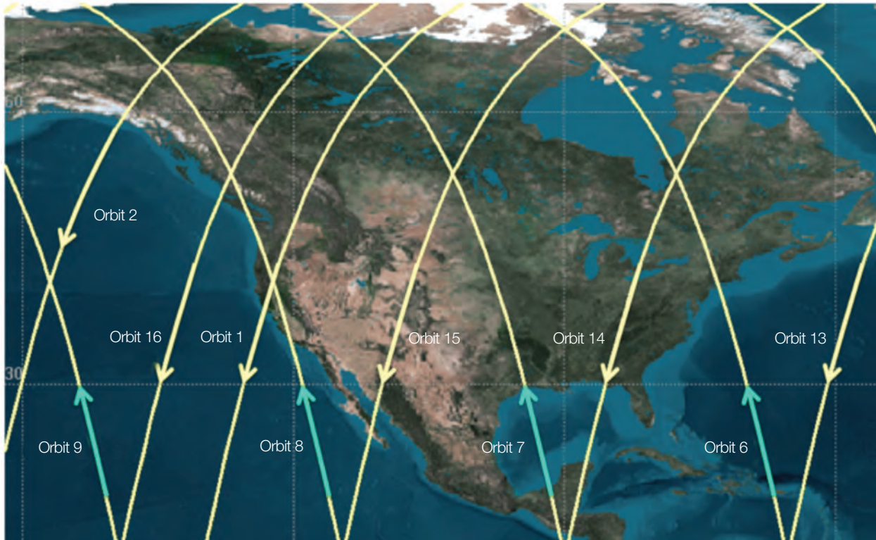
Figure 7. One-day ground track pattern over North America (Orbit 16 begins about 24.615 hours after Orbit 1).
