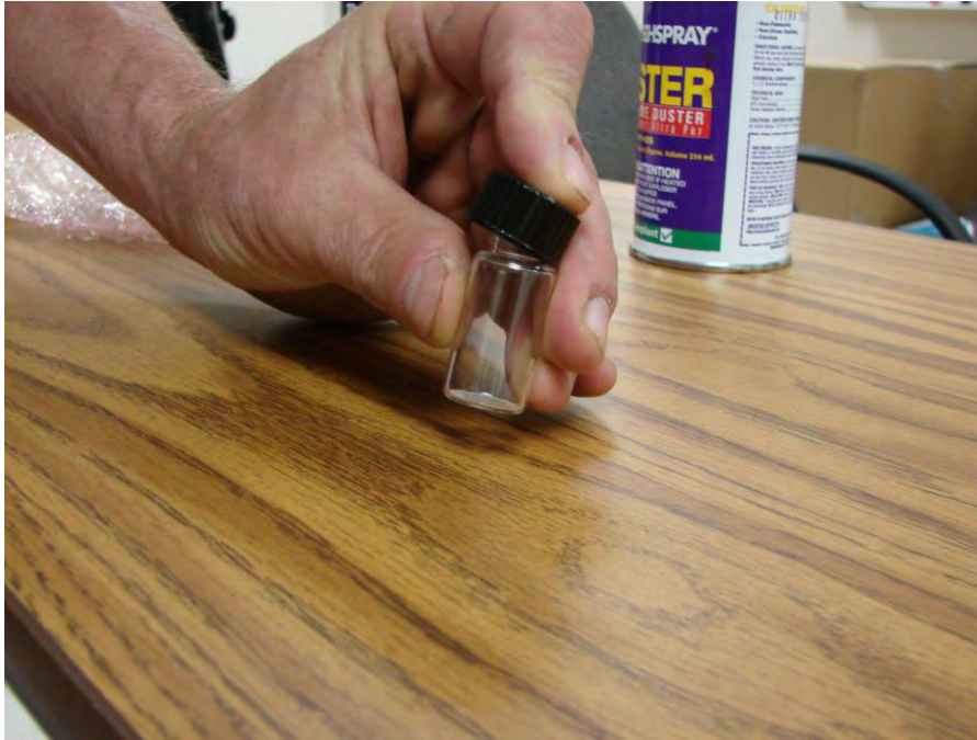
Figure 11: Tapping the Bead Dispenser to Dislodge Beads
