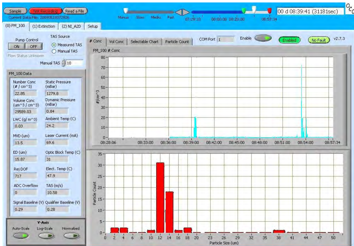
Figure 6: Display of Calibration Test Results. Note the definite peak in the 12-14 \mu\text{m} particle range.
