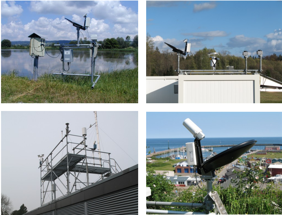
Figure 7: Examples of MRR installations
