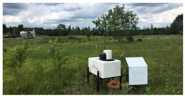
Figure 2: Halo Photonics Stream Line Doppler LiDAR at the CHEESEHEAD measurement campaign
