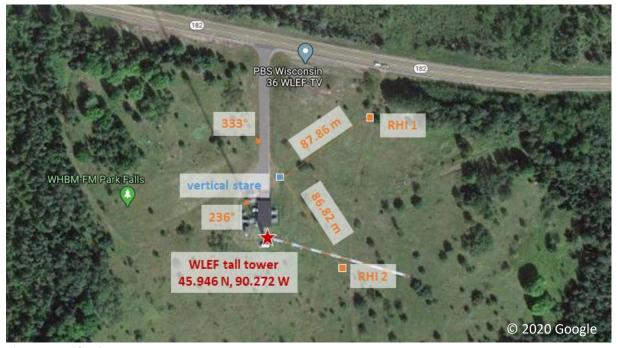
Figure 1: Doppler LiDAR setup
